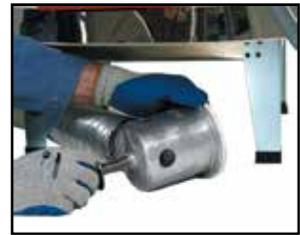
**STEP 6 - INSTALLING THE BLOWER AND MOTOR ASSEMBLY**
