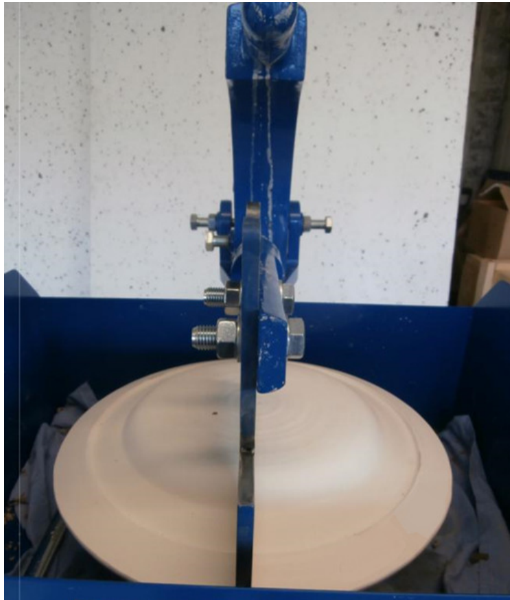
Photo showing Flat ware tool mounted from the front. Note: the tool mount has to be rotated to mount the flat ware tool on centre.
