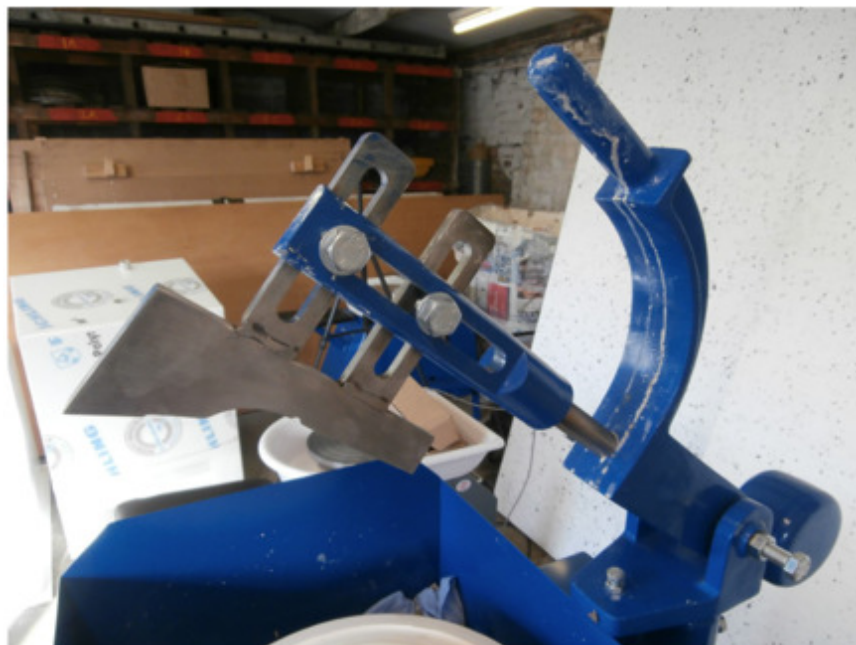
Photo showing flat ware tool mounted from the side, note the tool is mounted on the front edge of the mould.
