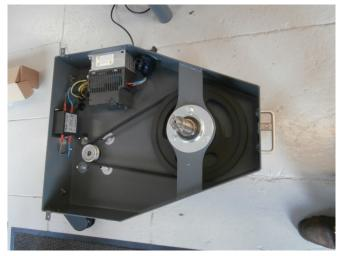
5) Release the cable gland securing the cable that goes to the foot pedal by undoing the dome top of the gland, it may be necessary to hold the gland body to prevent it from
