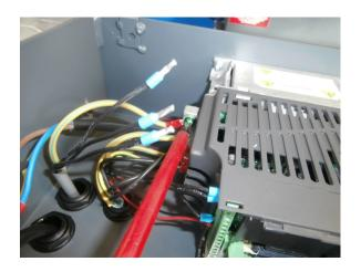
10) Attach the three pedal cables using the small flat head screw driver as indicated do not over tighten and then check they are secured by gently pulling on the cable.
