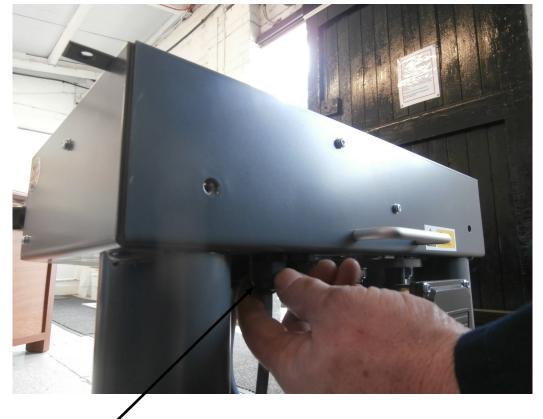
Dome top gland, ensure it is secured when reassembling.
