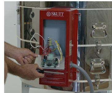
3. Switch the Red wires from your old control board to the Conversion Board. The terminal posts are labeled, but move one at a time to not mix them up.
