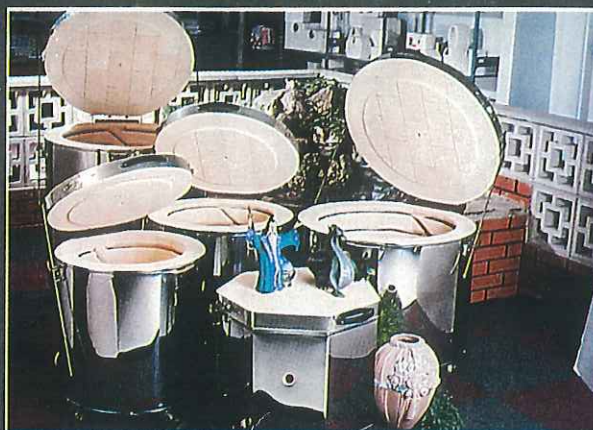
▲ Cluster of Cromartie Top Loaders equipped with brick lid. Note: All CTL kilns offer 76mm (3") fire brick.
